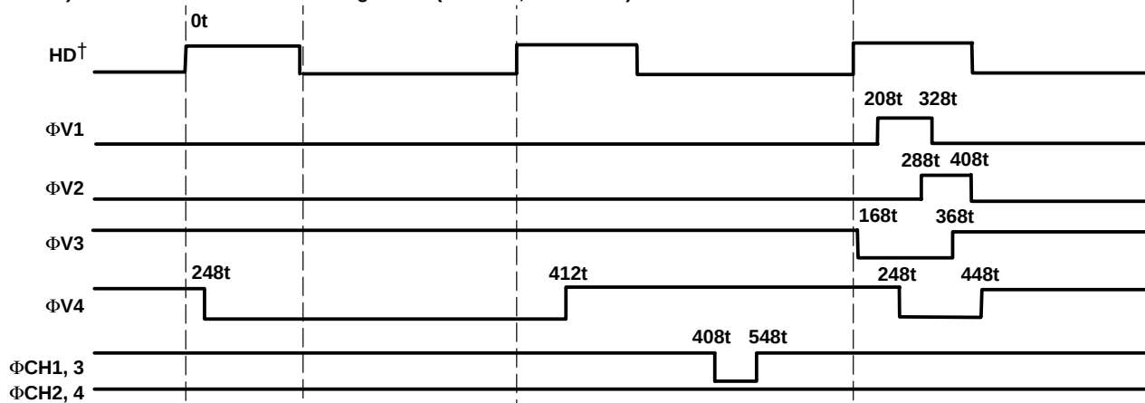
2) V-Rate Readout Detailed Timing Chart: ( \times 2 Mode, Even Field)
